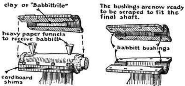
A dummy shaft must be used because the uneven heating by the babbitt metal might warp the finished shaft and ruin it.
