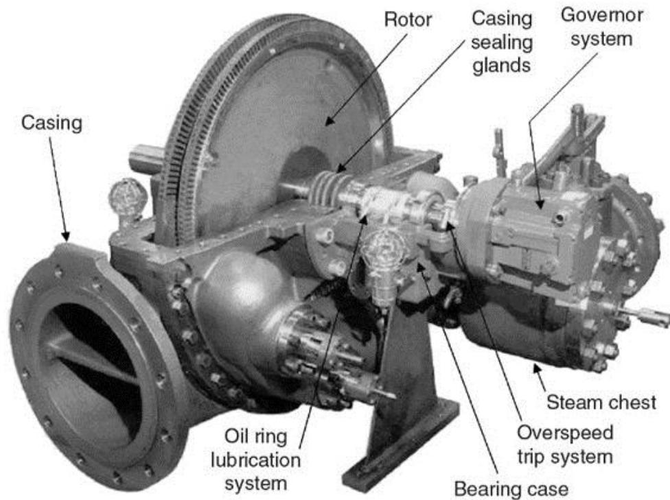
Single Stage Impulse Steam Turbine Cutaway
