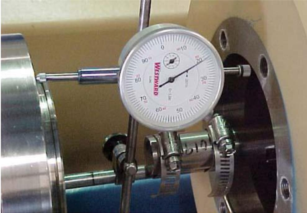
Coupling alignment using dial indicator method.
